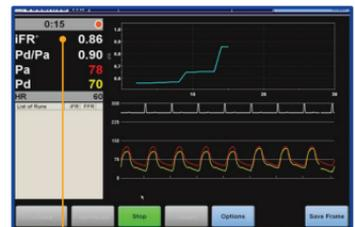
1. An iFR cut-point of 0.89 matches best with an FFR ischemic cut-point of 0.80 with a specificity of 87.8% and sensitivity of 73.0%. (iFR Operator's Manual 505-0101.23).
